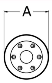
A = 208 D1 = 85 D2 = 85 L = 206 Nom. torque NM (Tkn) = 5000
